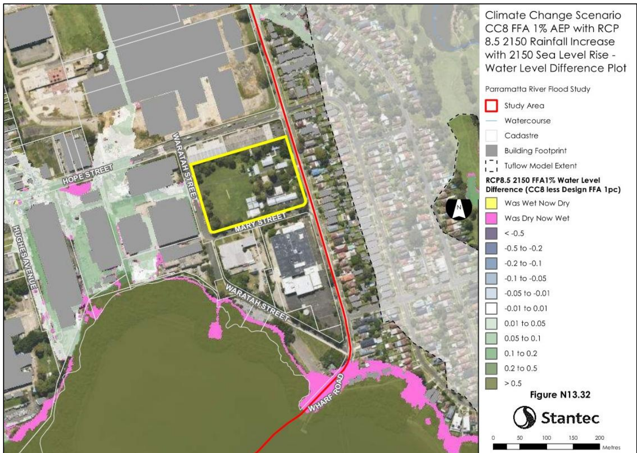
Figure 12: Impact of climate change (RCP8.5 in 2150) on flood levels and extents (Source: City of Parramatta, 2024)
