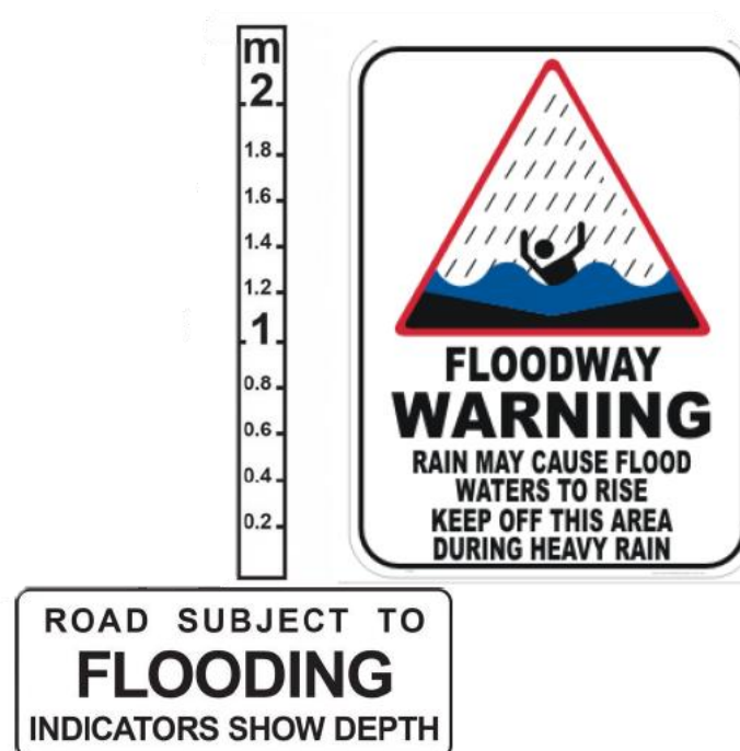
Figure 11: Signage and Gauges
